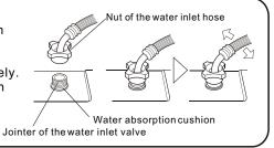
Note: The new hose-set supplied with appliance are to be used and the old hose-sets should not be reuse.
